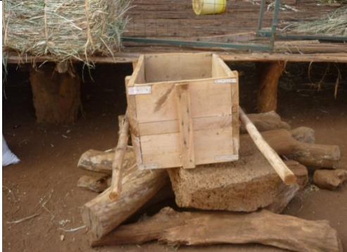
A wooden box for manually baling hay on-farm
