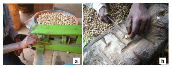
Plate 3.3: Extraction of Melia seeds from nuts using: (a) a Melia nut cracker and (b) knife
