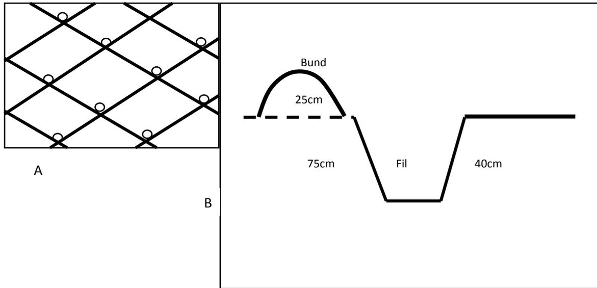
**Figure 1.** Micro-catchments in a plot (A) and a side view of bund and hole for trapping water in a micro-catchment (B)
