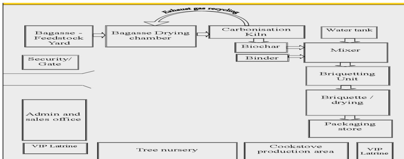
**Figure 2.** Schematic process flow of carbonized briquette production
