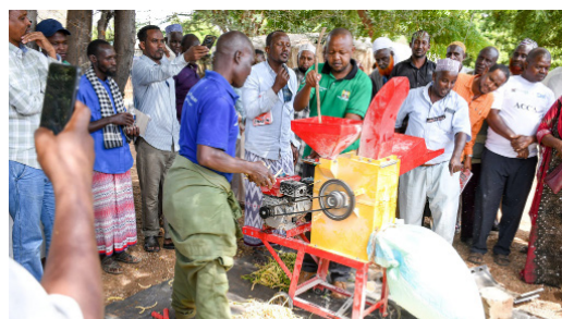
KEFRI staff Nathaniel Nyamai demonstrating the use of portable grinding machine to convert Prosopis pods to flour
